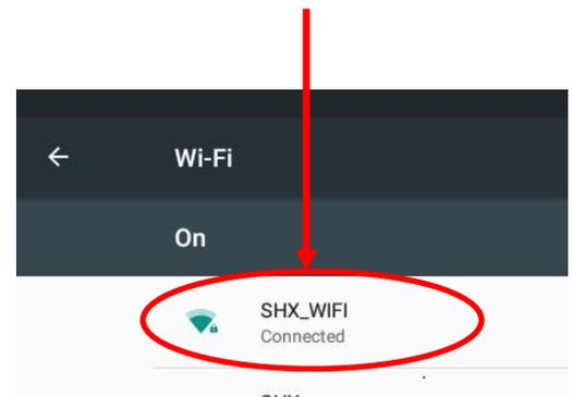
When the Tablet is connected to the Wi-Fi, it must be indicated with the Wi-Fi icon on the top right corner of the tablet:
