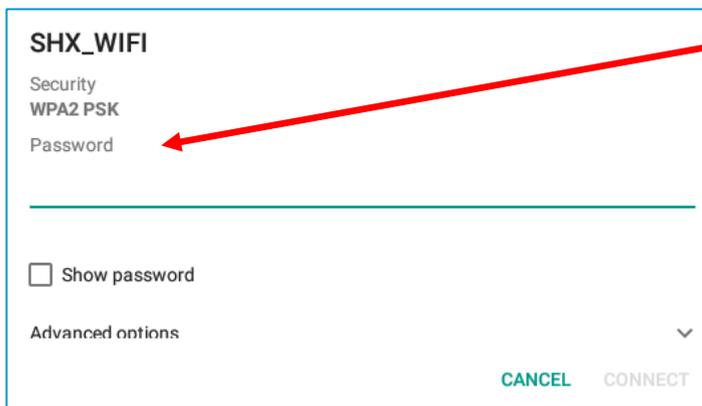
5. After selecting **SHX\_WIFI** it will be necessary to introduce the password. By default, the password is **TEmporal123456**.
