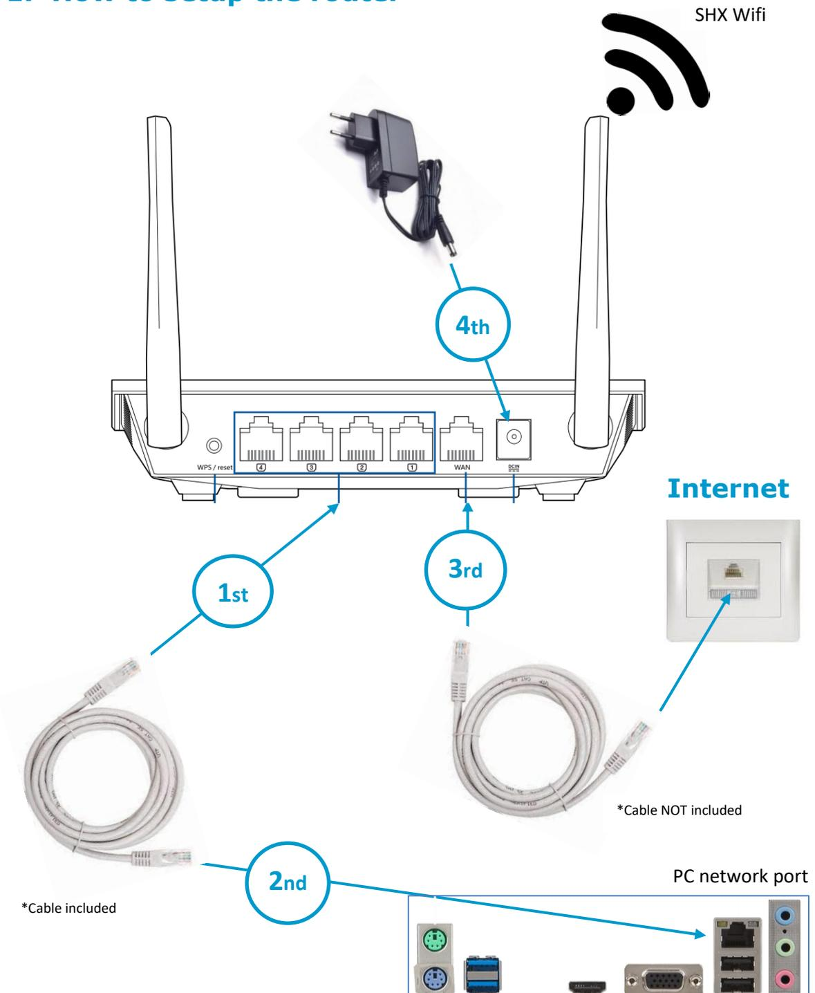
1. Connect the ethernet cable delivered with the product to any of the ports 1, 2, 3 or 4 of the router.
